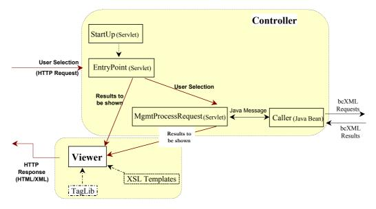
FIG. 9: Internal view of bcXB.
