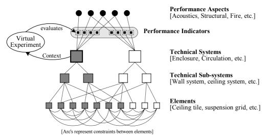
FIG. 11. Mapping between the functional system approach and performance concept.
