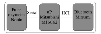
FIG. 6: The EIS test platform architecture. A sensor, in this case a pulse oxymeter, is serially connected to a microprocessor, Mitsubishi M16, running a real time operating system (RTOS) with appropriate parts of the "TCP/IP" suite of protocols and a host controller interface, HCI driver communicating with a Mitsumi Bluetooth 1.1 device.
