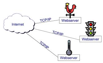
FIG. 2: Minimal Internet server architecture for ad-hoc connection of small devices like sensors connected to the Internet.
