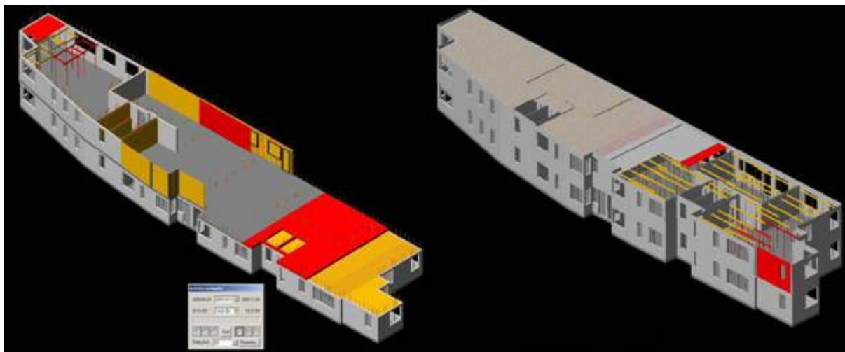
FIG. 5: Parallel simulation and comparison of construction alternatives in 4D CAD. (Left) Traditional production technology. (Right) Industrialized practice combining innovative technologies, such as permanent formwork systems, reinforcement carpets and self-compacting concrete. Colour settings in simulations: Red = in activity, grey = finished elements, yellow = traditional formwork and shoring elements
