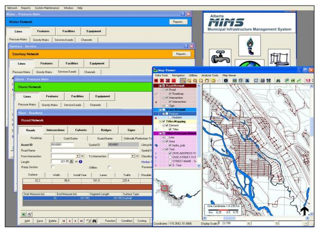
FIG. 3: MIMS main windows for managing water, sanitary, storm water, and road networks, each showing the break down of the network to primary components and asset types. The MapViewer is shown with a sample data (Courtesy of the MIMS Initiative).
