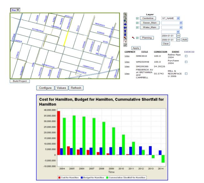
FIG. 4: View of RIVA showing GIS integration (Top) and long-term impact of infrastructure funding (Bottom).
