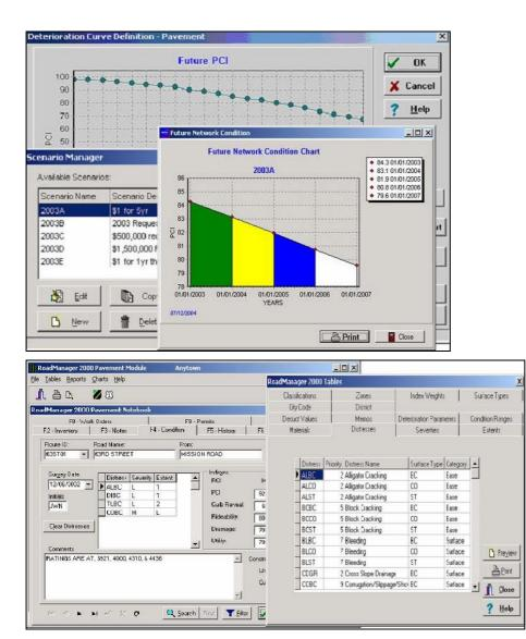
FIG. 6: Sample screens from RoadManager2000 showing the Pavement module notebook and table options, pavement assessment, and deterioration curves from the Budget Analysis module.
