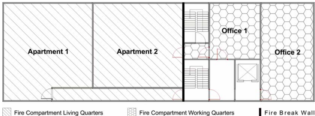
FIG. 11: Design of Fire Protection Elements.
