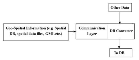
FIG. 3: Design of a data converter to integrate geo-spatial information with nD-modelling database
