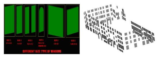
FIG. 10: Left, images of windows generated by BDIS; Right, 3D VRML model of just windows and doors in Jactin House
