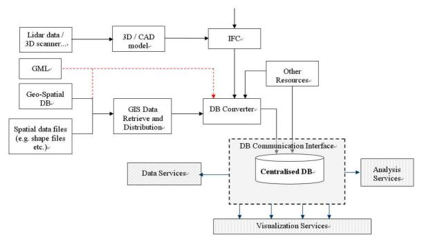
FIG. 4: BDIS top level data flow diagram
