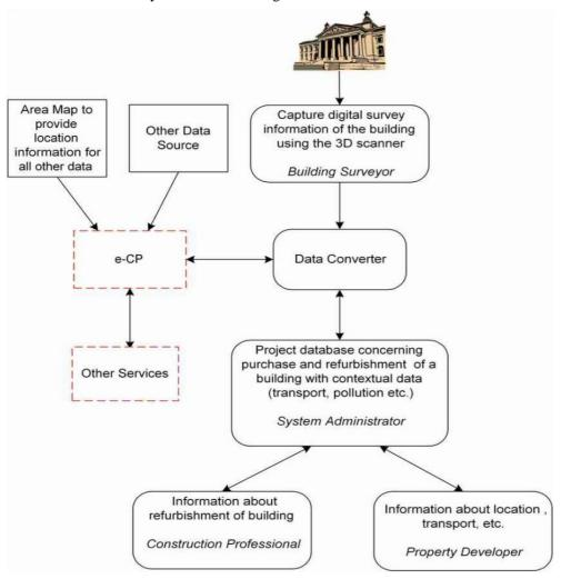
FIG. 1: Built environment Data Integration System showing main components and key actors
