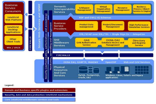
FIG. 6: InteliGrid high-level platform components.
