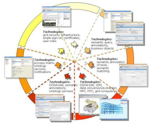
FIG. 11: Generic InteliGrid end user scenario presented with different application screenshots and relevant technologies.
