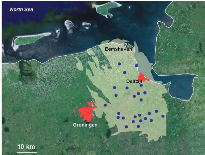
FIG. 48. Northern part of The Netherlands with the towns Groningen and Delfzijl. The light green area is the Groningen gas-field. Locations of gas production units (so called clusters) are marked with blue dots.
