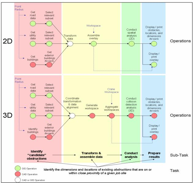
CAD) must be manually matched to the global coordinate system used by the GIS; on the other hand, in the 3D approach, the global coordinate system of existing structures within the GIS need to be transformed into the local referencing system used within the CAD.
