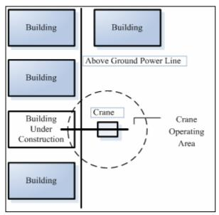
FIG 1: Potential obstructions for a crane based on its workspace
