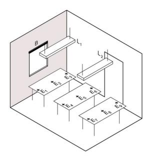
FIG.11: Schematic illustration of the test bed with the two luminaires (L1, L2), the shading device (B), and the workstation with reference points (E1, E2, E3) for workstation illuminance
