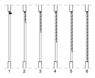
FIG.12: Illustration of the six discrete control states of the shading device in the test bed
