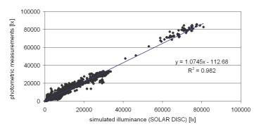
FIG. 3: Comparison of measured external illuminance levels with corresponding camera-based values
