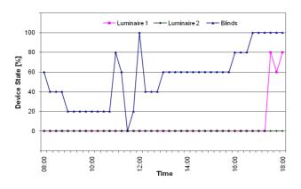
FIG.13: Recommendations (desirable states of lighting and shading devices) of the simulation-assisted lighting and shading control system for a reference day
