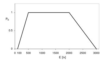
FIG. 15: Illustration of the assumed preference function for workstation illuminance
