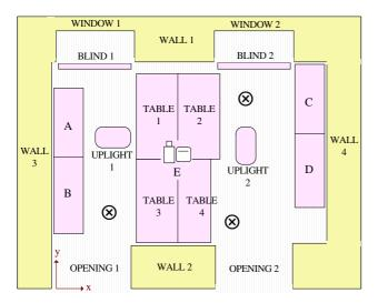
FIG. 4: Plan of the test-bed ("A" to "D" refer to Cabinets; "E" refers to Camera)
