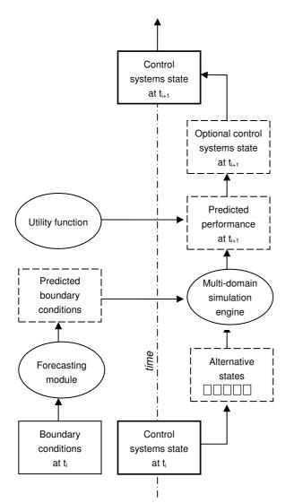
FIG. 1: The schematic illustration of a simulation-assisted building systems control strategy
