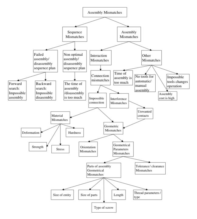
FIG 2: A Taxonomy for Parts of Assembly Adapted from Taratoukhine and Bechkoum (2000)
