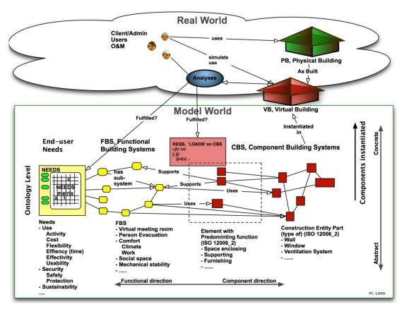
FIG. 3: Formalisation of the building design process. References are made to (ISO 12006-2, 1001) from (Christiansson et al, 2009b). Performance check and evaluation of solutions (the analyses round box) are made on both qualitative and quantitative performance criteria.
