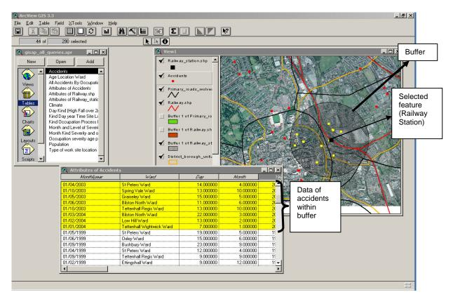
FIG 11: Example - Buffer around a Specific Feature
