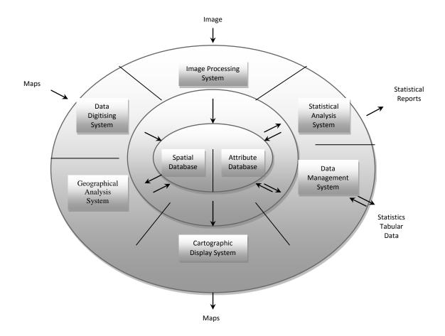
FIG 2: Software Components of a GIS Source: Eastman et al (1993)
