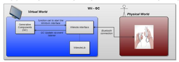
FIG 5: The software architecture of the Wiimote-GC experiment
