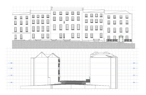
FIG. 22: Automated 2D documentation from BIM model.
