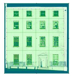
FIG. 17: Orthographic image overlaid with parametric façade template for graphical editing of façade elements.
