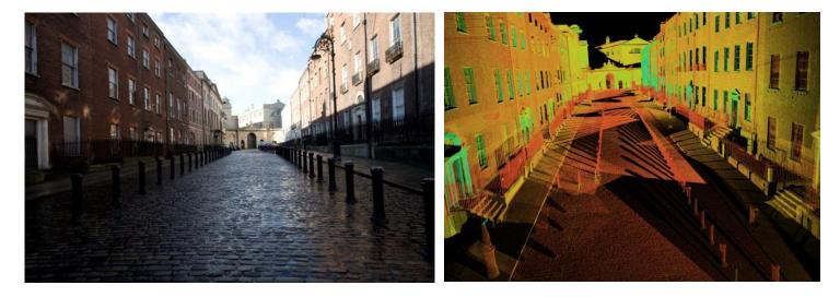
FIG. 20: Henrietta Street, Dublin (left) and point cloud of street coloured by intensity (right).
