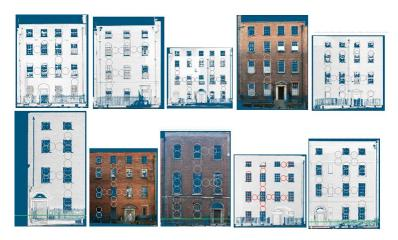
FIG. 3: Testing classical proportions using orthographic images from surveyed classical buildings.
