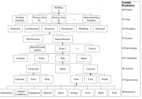
FIG. 5: Example WBS of a building project
