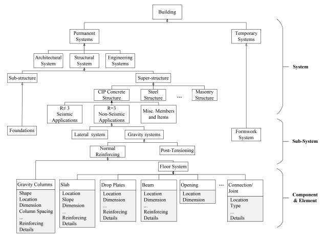
FIG. 4: Example product information architecture of Building A with Cast-In-Place Concrete Structure
