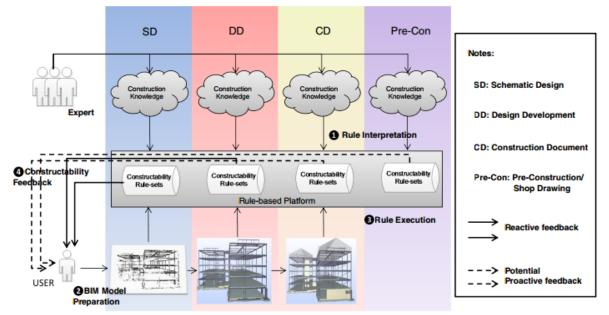
FIG. 2: Rule-based constructability checking (Jiang and Leicht, 2014)
