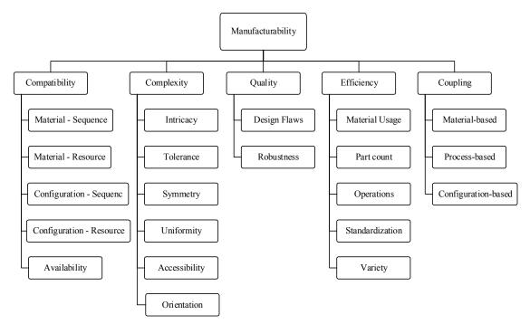
FIG. 1: A hierarchical model of manufacturability concepts (adapted from Shankar, 1993)
