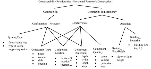
FIG. 10: Validated constructability links with required design information to support decision making of horizontal formwork systems in this case study
