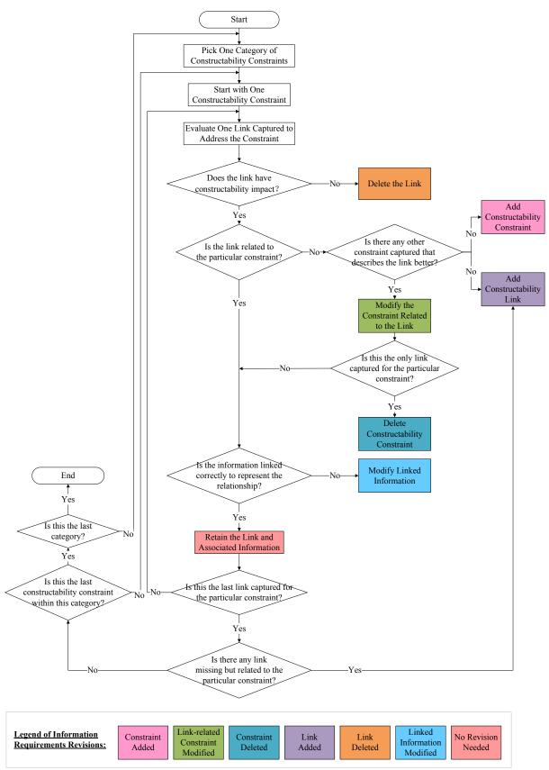
FIG. 9: Validation procedures of constructability links and information requirements
