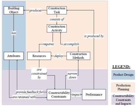
FIG. 3: An object-oriented representation of the ontology of a constructability review
