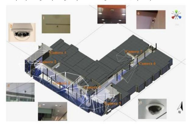
Figure 11: BIM model aligned with FOVs in the game engine
