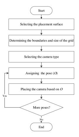
Figure 6: Placing camera using 2D grid
