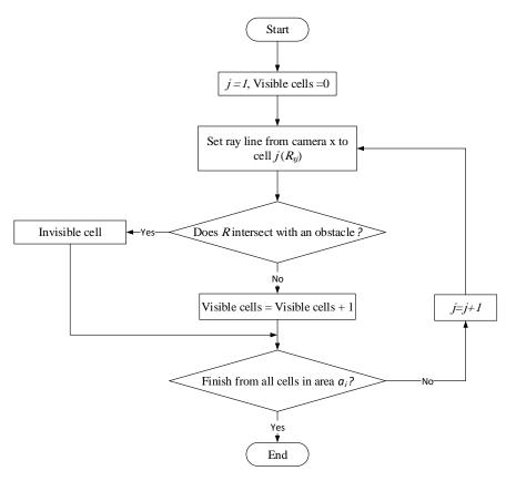
Figure 9: Camera visibility analysis in area  $a_i$
