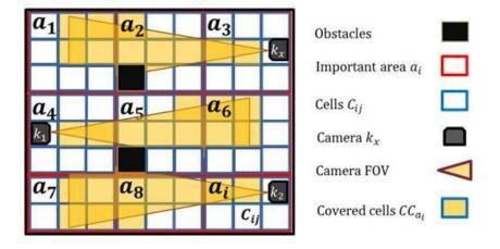
Figure 10: Example of coverage calculation (adapted from Albahri and Hammad, 2015)
