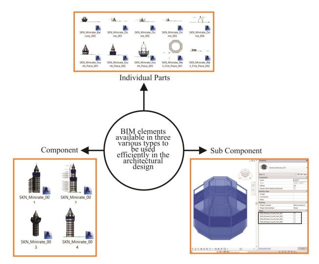
FIG. 11. BIM components in the digital library.
