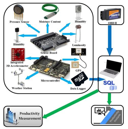
Figure 13: The Architecture of the Proposed Customized Data Acquisition System
