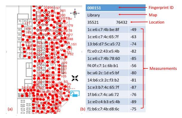
FIG. 2: (a) Fingerprints created in a building; (b) Attributes of a fingerprint
