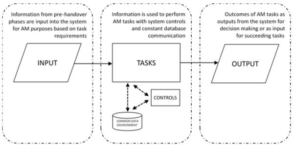
Figure 6: BIM-based AM Input-Output system
