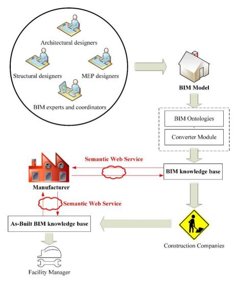
FIG. 1: Using Semantic Web Services (SWS) to integrate manufacturer product data with the BIM data.
