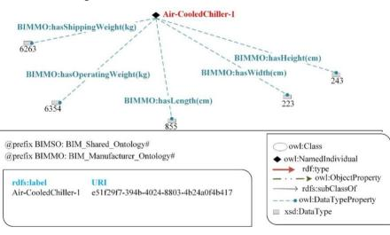
FIG. 15: A chiller's weight and dimensions
