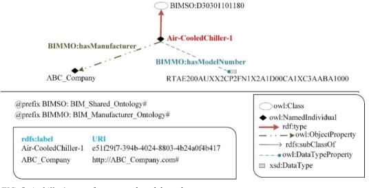
FIG. 5: A chiller's manufacturer and model number
