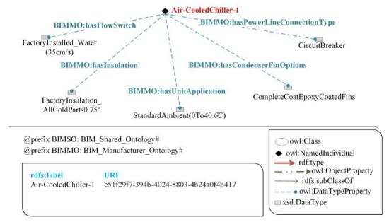
FIG. 9: A chiller's flow switch, insulation, unit application, condenser fin options, and power line connection type
