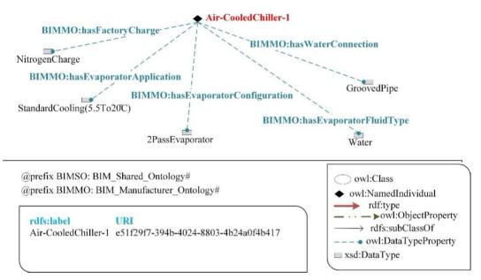
FIG. 8: A chiller's factory charge, evaporator application, evaporator configuration, evaporator fluid type, and water connection
