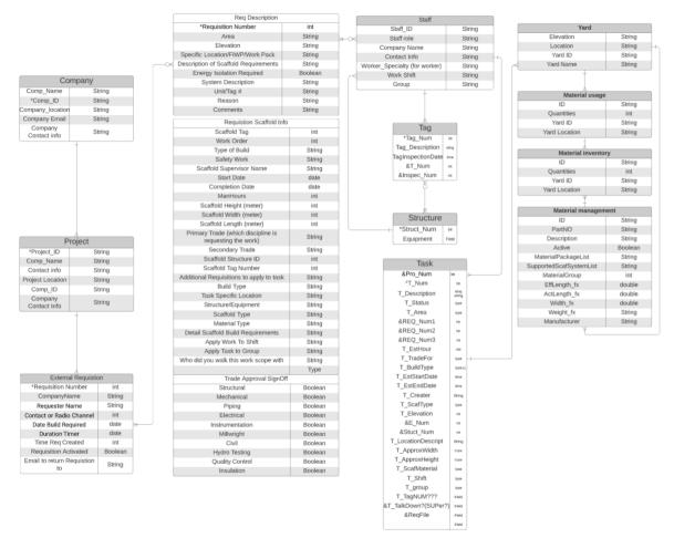
FIG. 5: Sample proposed entity relationship diagram of scaffolding management system.
