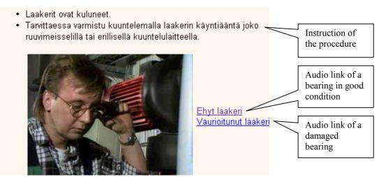
FIG. 5: A procedure for checking the condition of pump bearings using audio recordings.
