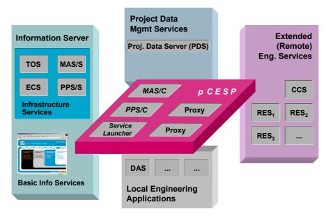
Fig. 6: Allocation of the components on the five domains of the full ISTforCE architecture.
