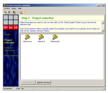
Fig. 15: Project selection through the GUI of the Service Launcher. The main Launcher frame dynamically creates references to the projects relevant to the logged in user.
