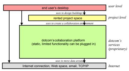
Fig. 3: Typical current architecture of services for engineers on the Web.
