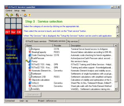
Fig. 16: Service selection through the GUI of the Service Launcher. Only services available to the logged in user
