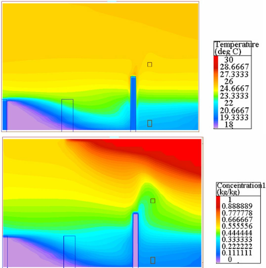
FIG. 23: Top: Temperature distribution in the  $xy$  symmetry plane of the displacement ventilated room (stratified flow field). Bottom: Concentration distribution in the symmetry plane in case of a warm point contaminant source. The concentration is made dimensionless, thus, it corresponds to the exhaust concentration. If the room was fully mixed the value would be 1 for the entire room.
