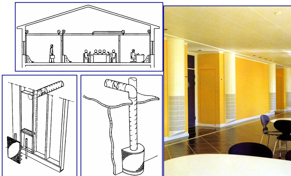
*FIG. 19: Application of displacement ventilation system. Left: Sketch of a solution including occupants. Below is shown details indicating how the inlet devices can be build in. Right: Photo of application in real life. Courtesy of Lindab A/S Denmark.*
