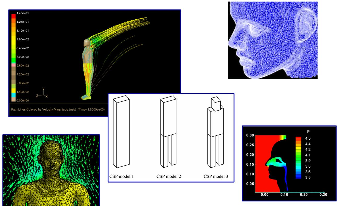
FIG. 3: Virtual models of persons, Computer Simulated Persons (CSP) with different level of detail used to study airflow around persons and personal exposure (Brohus, 1997). [Click here for video animation of the lower left figure.](#)
