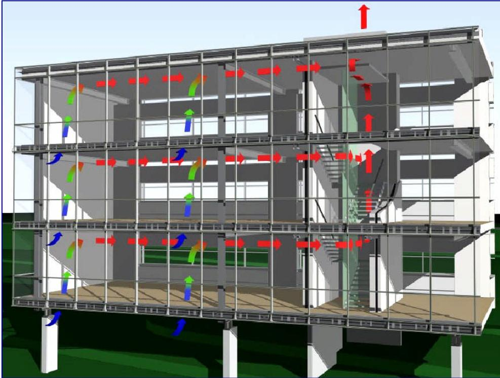
*FIG. 25: Outline of airflow in B&O HQ building. Courtesy of Birch & Krogboe, Consultant Engineers, Denmark.*
