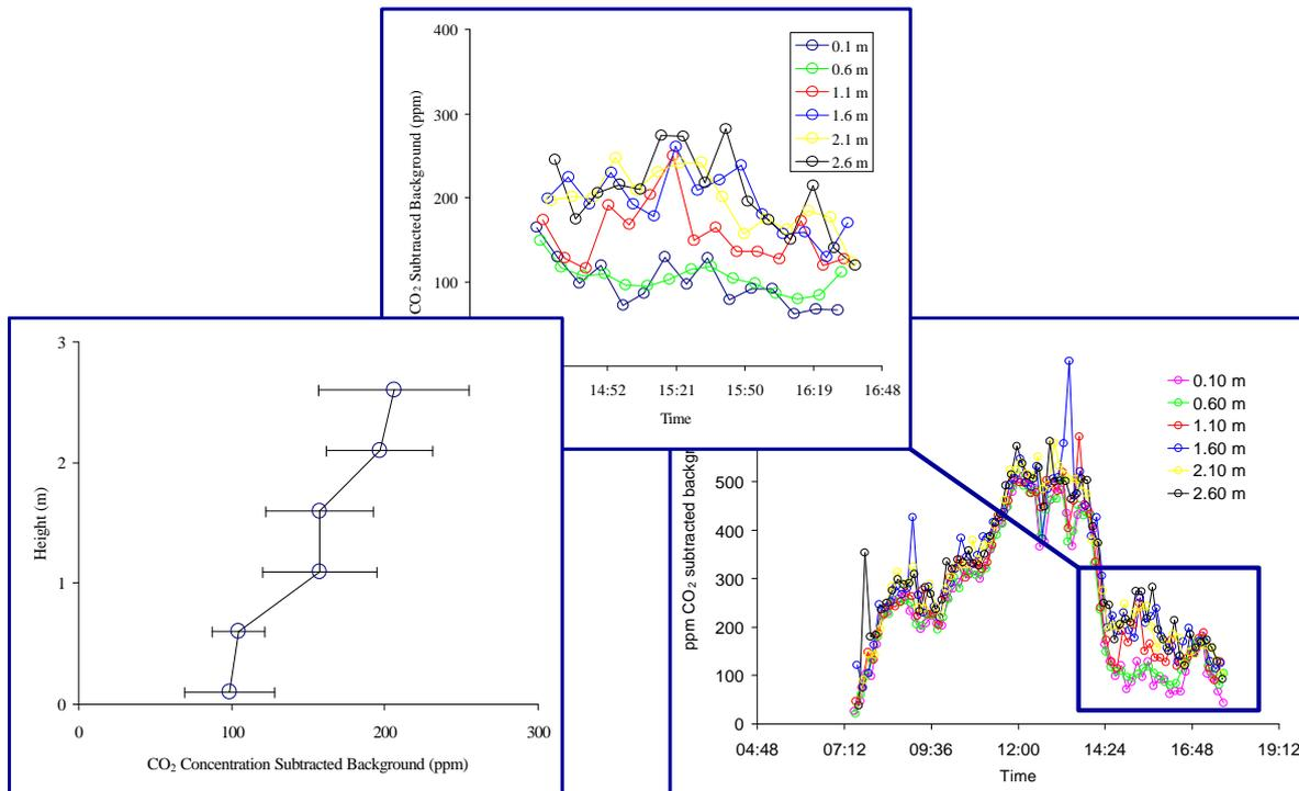
FIG. 27: Results from concentration measurements. CO<sub>2</sub> measurements are performed at different heights in the displacement ventilated open plan office at the B&O building. Further treatment of data indicates relatively high ventilation effectiveness as assumed in theory and qualitatively suggested in Fig. 25. For further details, see (Brohus et al., 2003).
