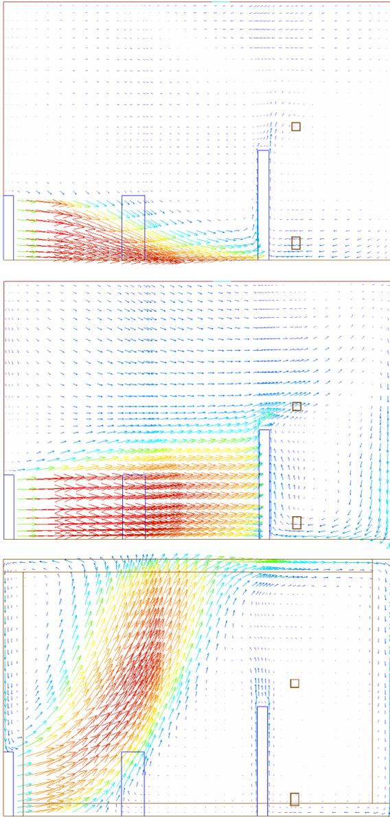
FIG. 22: Influence of supply air temperature in displacement ventilated room (xy-plane). Visualisation of the influence of the supply air temperature compared with the room air. Top: Cold supply air. Centre: Isothermal supply air (same temperature as the room air). Bottom: Warm supply air (See Fig. 20 for geometry details).
