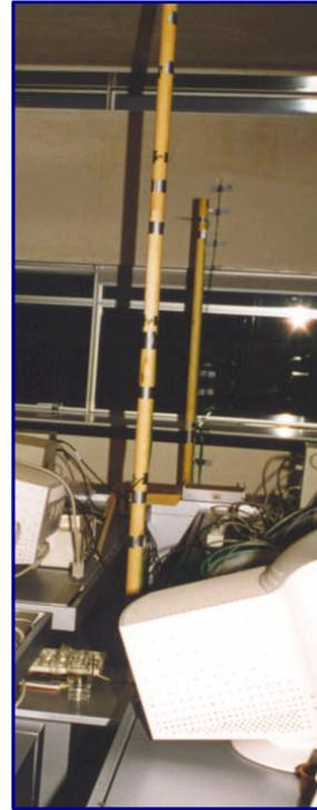
FIG. 26: Measurement equipment applied for the tracer gas measurements at the B&O building. The measurements are used to verify and quantify the airflow suggested in Fig. 25.
