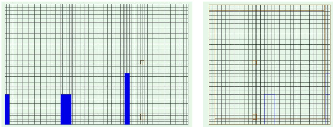
FIG. 21: Computational grid applied in the CFD simulations. Left: xy-plane, right: zy-plane
