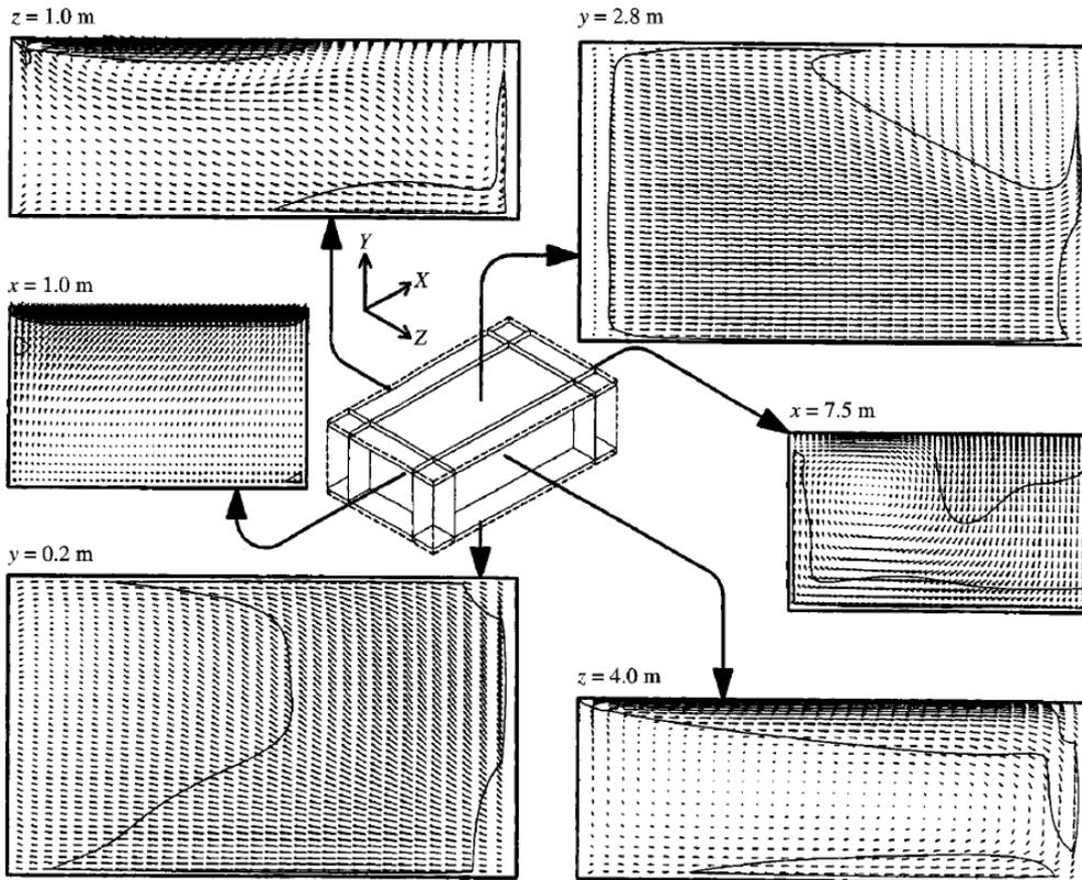
FIG. 4: Three-dimensional airflow simulation results illustrated by a number of two-dimensional plots (Bjerg et al., 1999)
