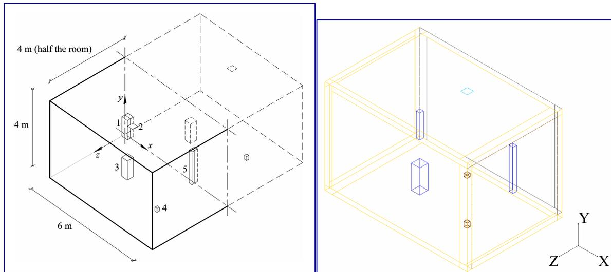
FIG. 20: Left: Geometry of displacement ventilation CFD test case. The subcooled air is supplied by a low-velocity inlet device (1) and it is exhausted through two return openings in the ceiling (2). The heat load is generated by two person simulators (3), a point heat source (4) and a Computer Simulated Person (CSP) (5), represented by a heated cuboid. Right: Outline of case in computational tool.
