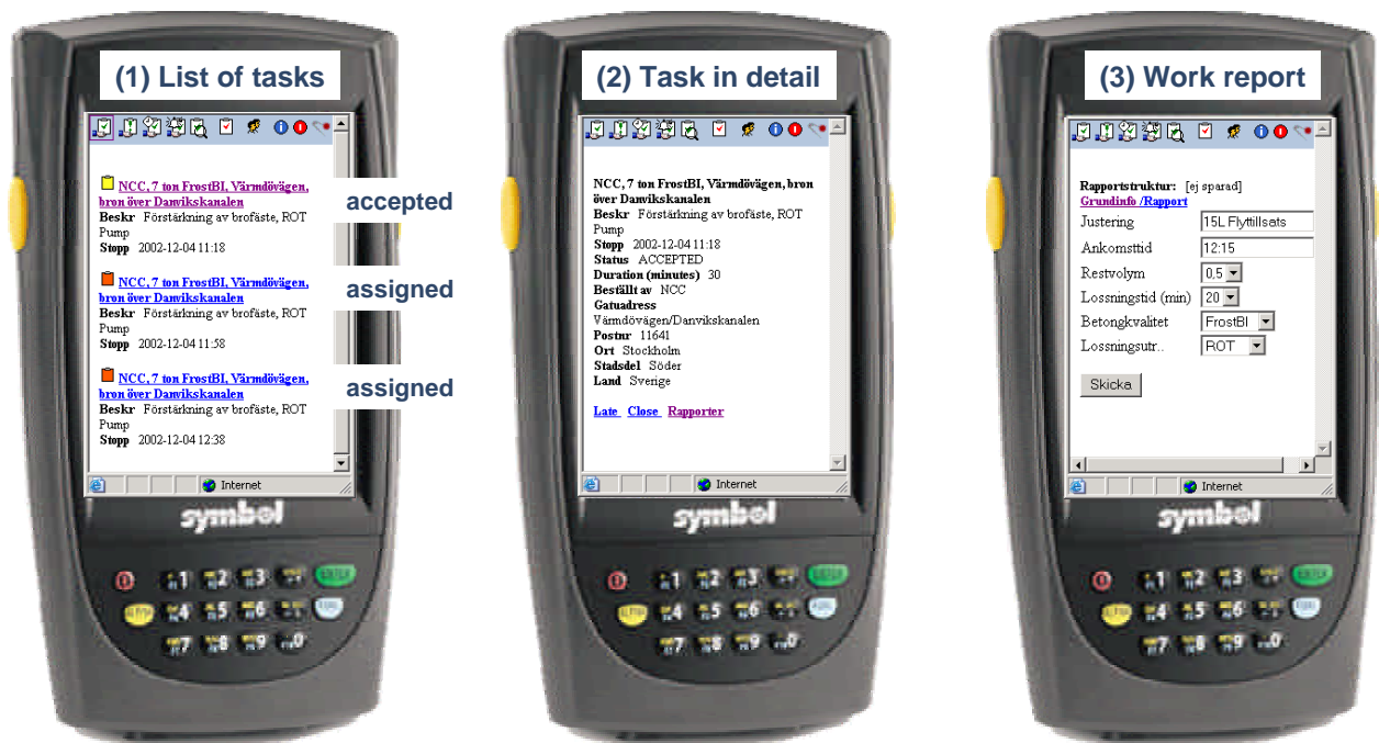
FIG. 3: Field worker interface for concrete delivery. (1) List of accepted (yellow) and assigned (red) tasks, (2) order in more detail and (3) work report upon completed task.
