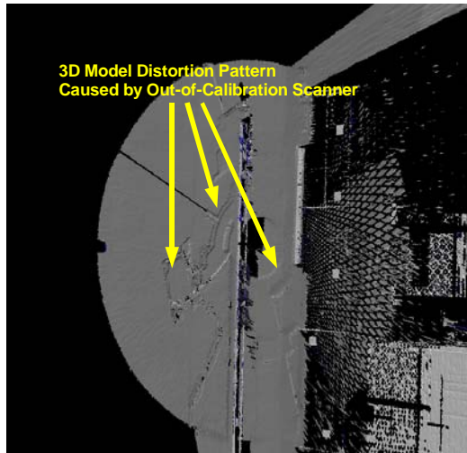
FIG 4: Geometric distortion patterns caused by a scanner that is not calibrated observed in Case 6.
