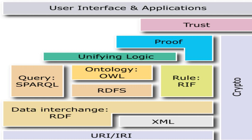
FIG. 3: The Semantic Web architecture (source: W3C, 2008)
