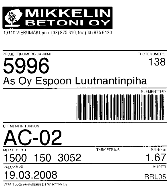
FIG. 3: Coated paper label with 1D barcode of an element identifier.
