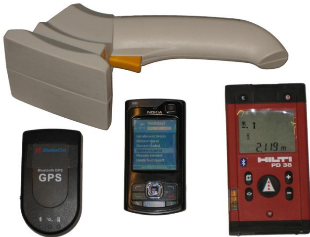
FIG. 7: Mobile phone, RFID-reader, GPS receiver and laser dimension meter.
