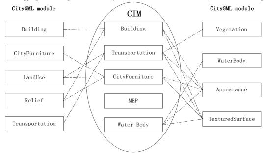
Figure 7: The mapping relationship between cityGML and CIM
