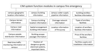
Figure 9: CIM system function modules in campus fire emergency
