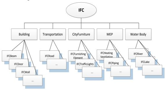
Figure 8: The mapping relationship between IFC and CIM
