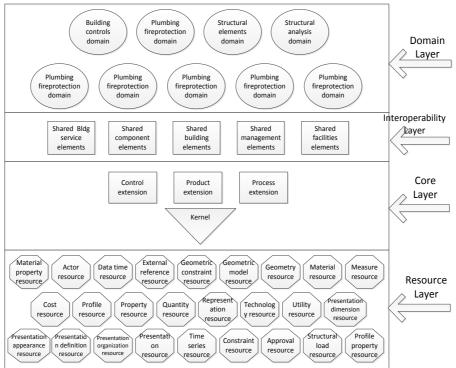
Figure 3: IFC schema
