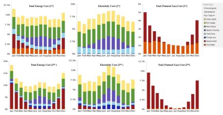
FIG. 9: Monthly cost analysis results for Total Energy, Electricity and Fuel (Natural Gas) for two design options
