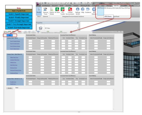
FIG. 5: Snapshot of DSS plug-in developed in Autodesk Revit
