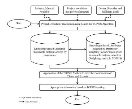
FIG. 3: Decision Support System Schema using TOPSIS algorithm
