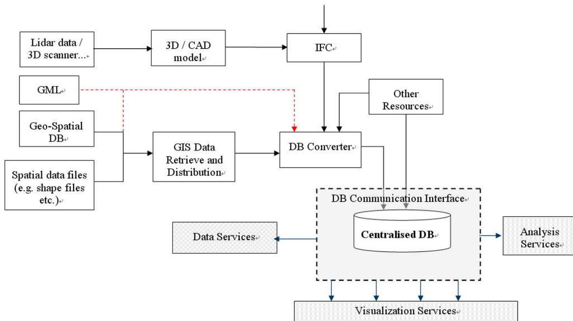
FIG. 4: BDIS top level data flow diagram
