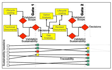
FIG. 1: Requirement-based integrated design framework
