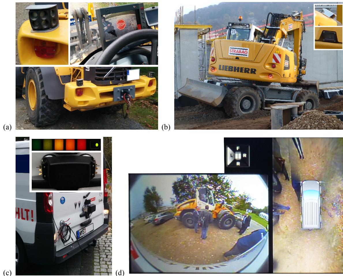
FIG. 2: Examples of real-time pro-active obstacle detection and alert technologies that do not automatically recognize persons: (a) sonar, (b) side- and rear-view vision cameras, (c) RADAR and (d) 360° surround view vision cameras (Teizer et al., 2015a)
