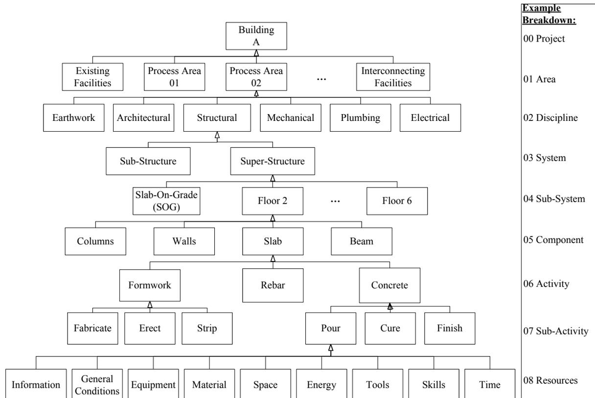
FIG. 5: Example WBS of a building project
