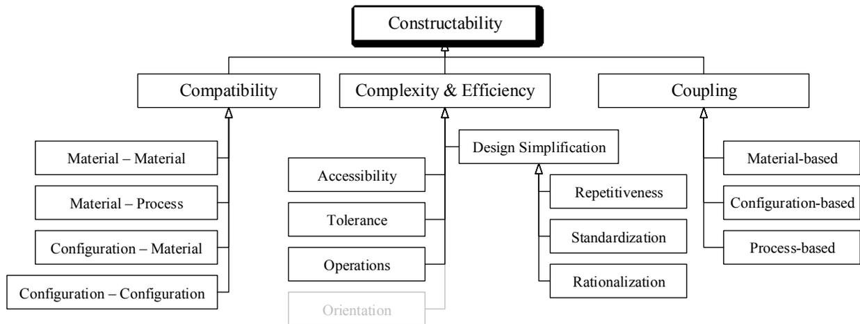
FIG. 6: A hierarchy model of constructability constraints
