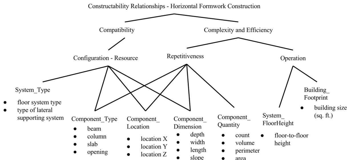
FIG. 10: Validated constructability links with required design information to support decision making of horizontal formwork systems in this case study
