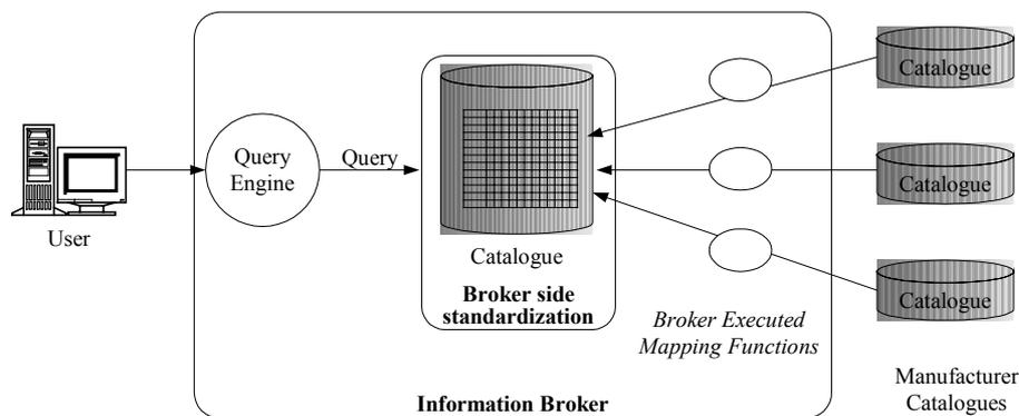
FIG. 5. Broker side standardization.
