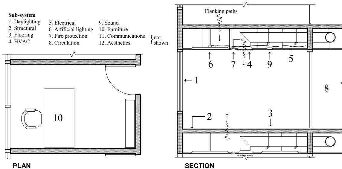
FIG. 10. Configuration of a typical office space used in the example.
