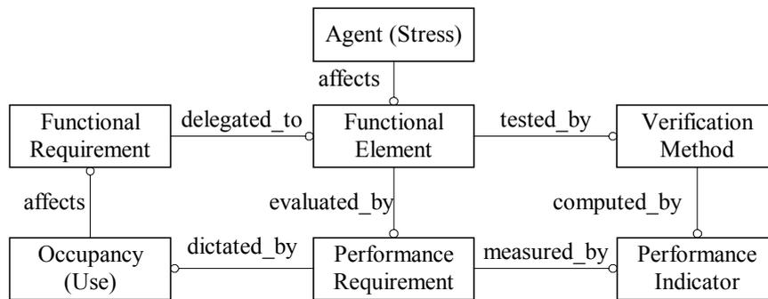
FIG. 8. Relationship among concepts in the performance approach. (Adapted from (Vanier et al., 1996)).
