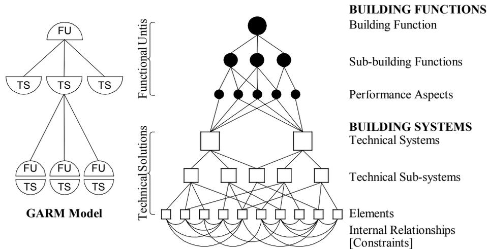
FIG. 7. Overview of a functional systems approach for product selection.
