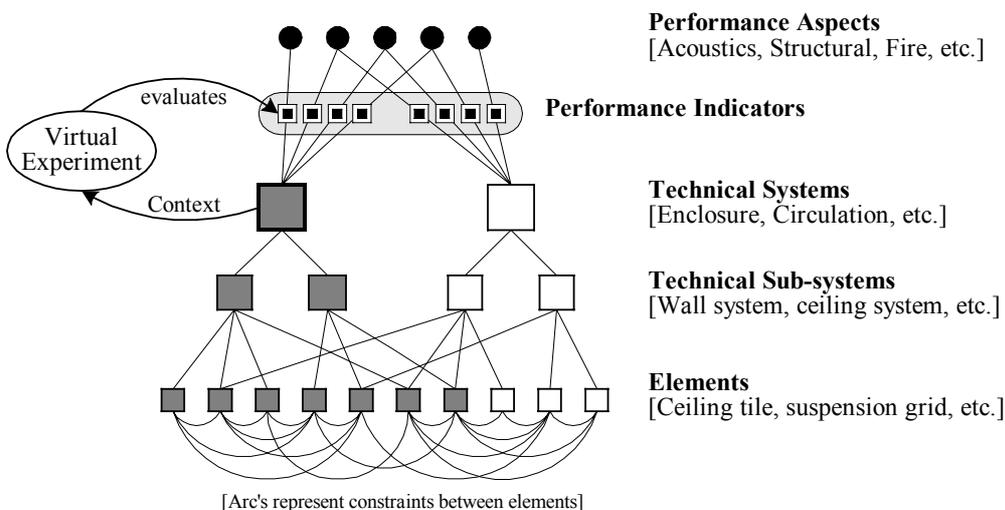
FIG. 11. Mapping between the functional system approach and performance concept.
