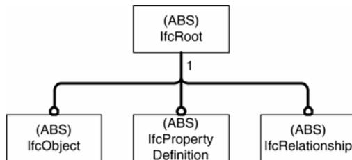
FIG. 6: The IFC "template model"
