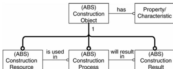
FIG. 2: The high level process model in ISO 12006-2.
