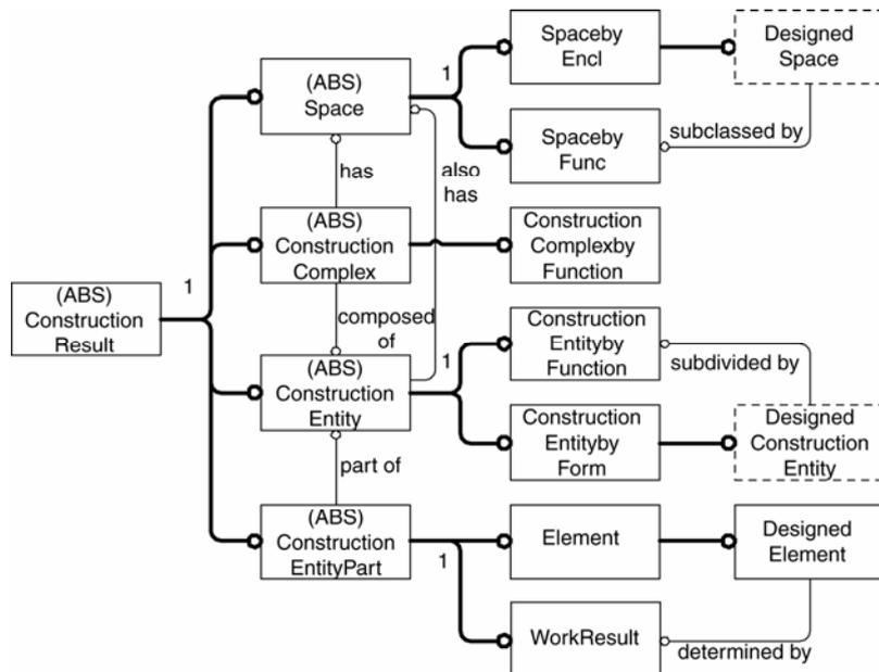
FIG. 5: Construction Result according to ISO 12006-2
