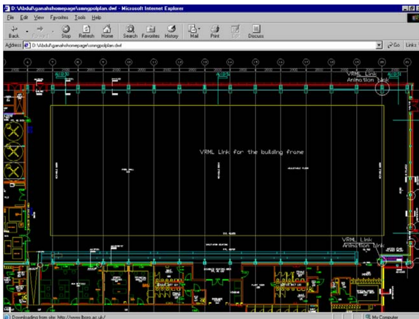
FIG. 8: 2D plan for the swimming pool with hyperlinks to VRML models and 3D animations
