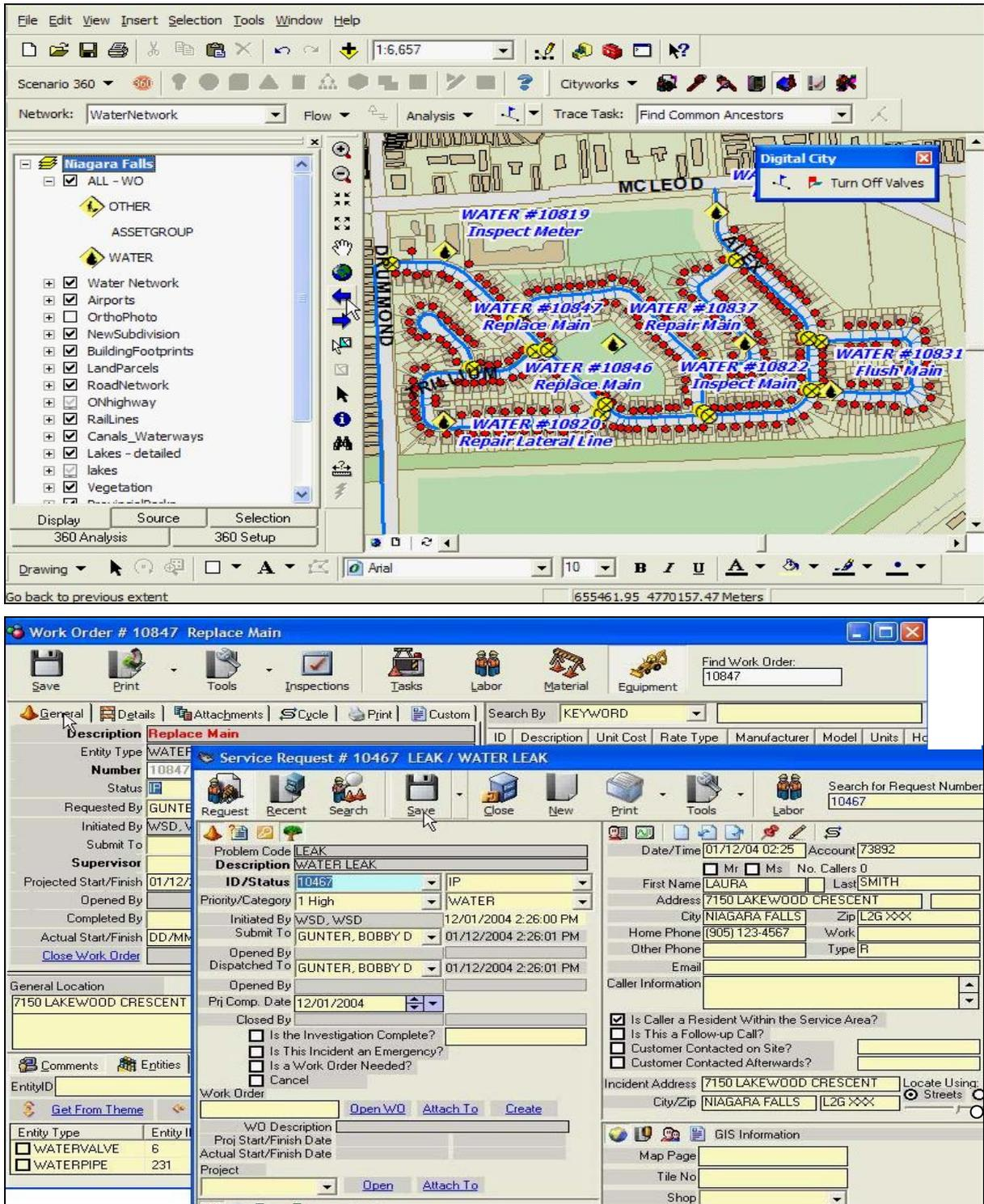
FIG. 2: (Top) CityWorks ArcGIS add-on showing a map of water mains and associated work orders; (Bottom) Forms for Work Order and Service Requests (Courtesy of Azteca).
