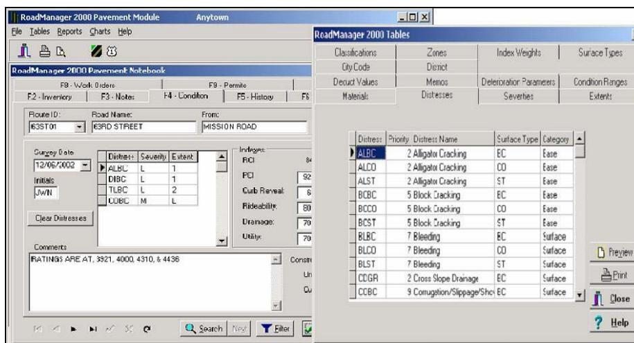
FIG. 6: Sample screens from RoadManager2000 showing the Pavement module notebook and table options, pavement assessment, and deterioration curves from the Budget Analysis module.
