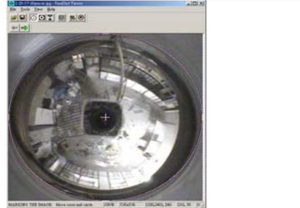
Image de-warp: A frame of map image is snapped and de-warped into panorama image to create a VR scene.
