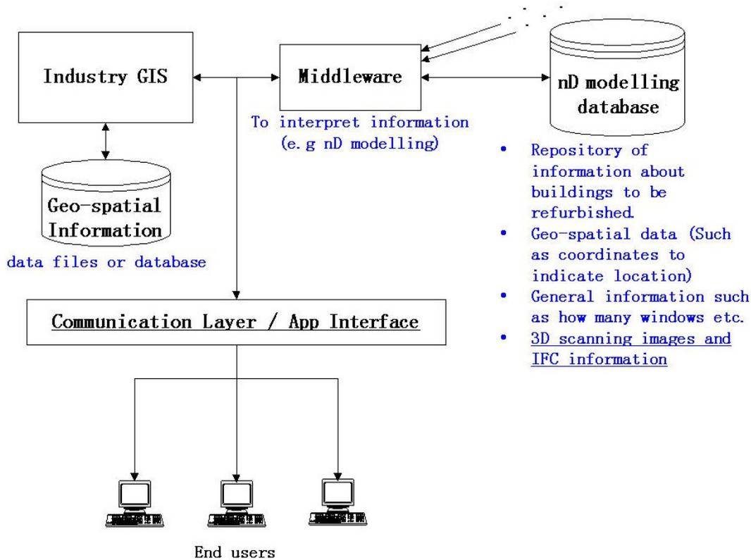
FIG. 2: Linking GVIS with an nD database using the communication layer
