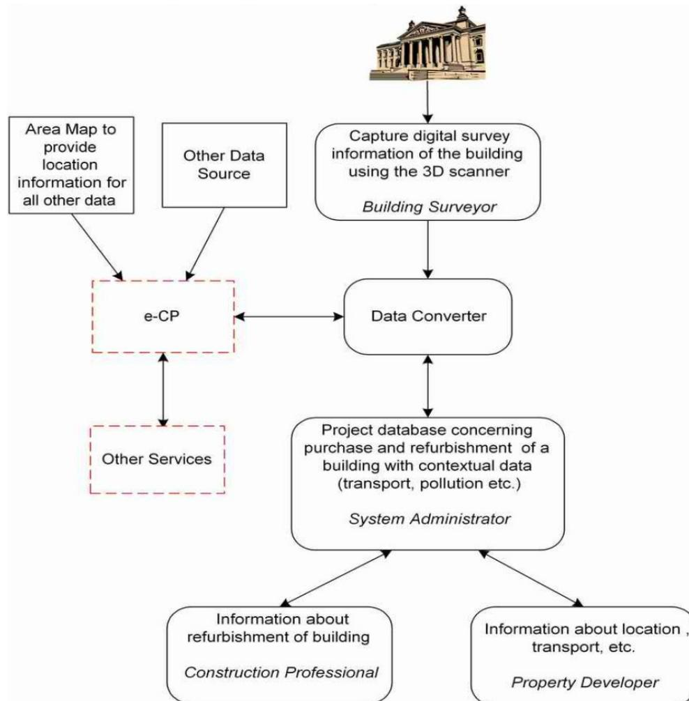
FIG. 1: Built environment Data Integration System showing main components and key actors
