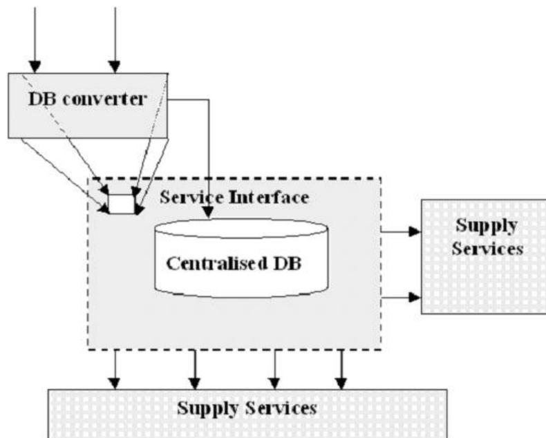
FIG. 12: The data converter forms part of the database service interface
