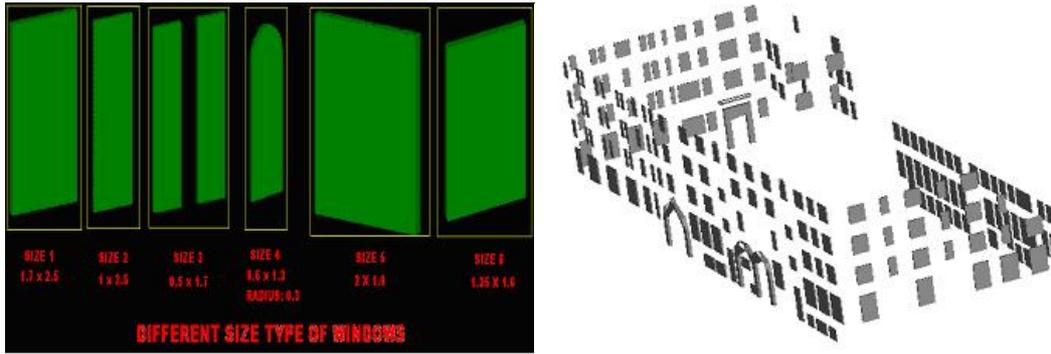
FIG. 10: Left, images of windows generated by BDIS; Right, 3D VRML model of just windows and doors in Jactin House
