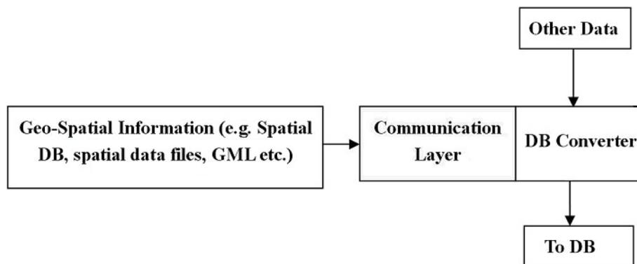
FIG. 3: Design of a data converter to integrate geo-spatial information with nD-modelling database
