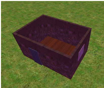
FIG. 1: An example of a design composition of a room using the assembly hierarchy architectural objects including walls, windows, doors and floor.
