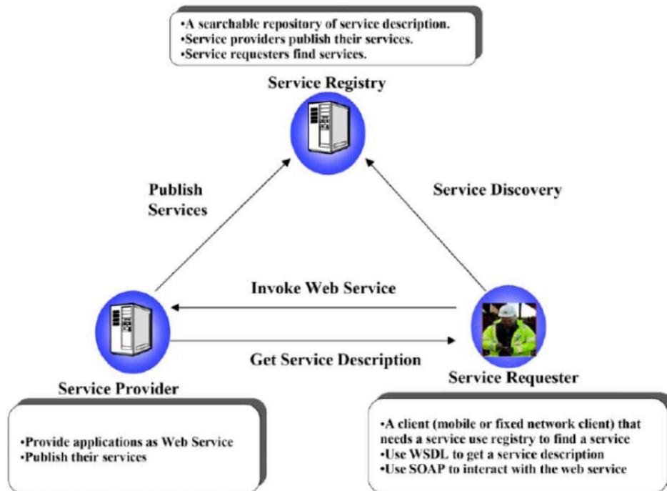
FIG. 4: Key components of Web Service architecture
