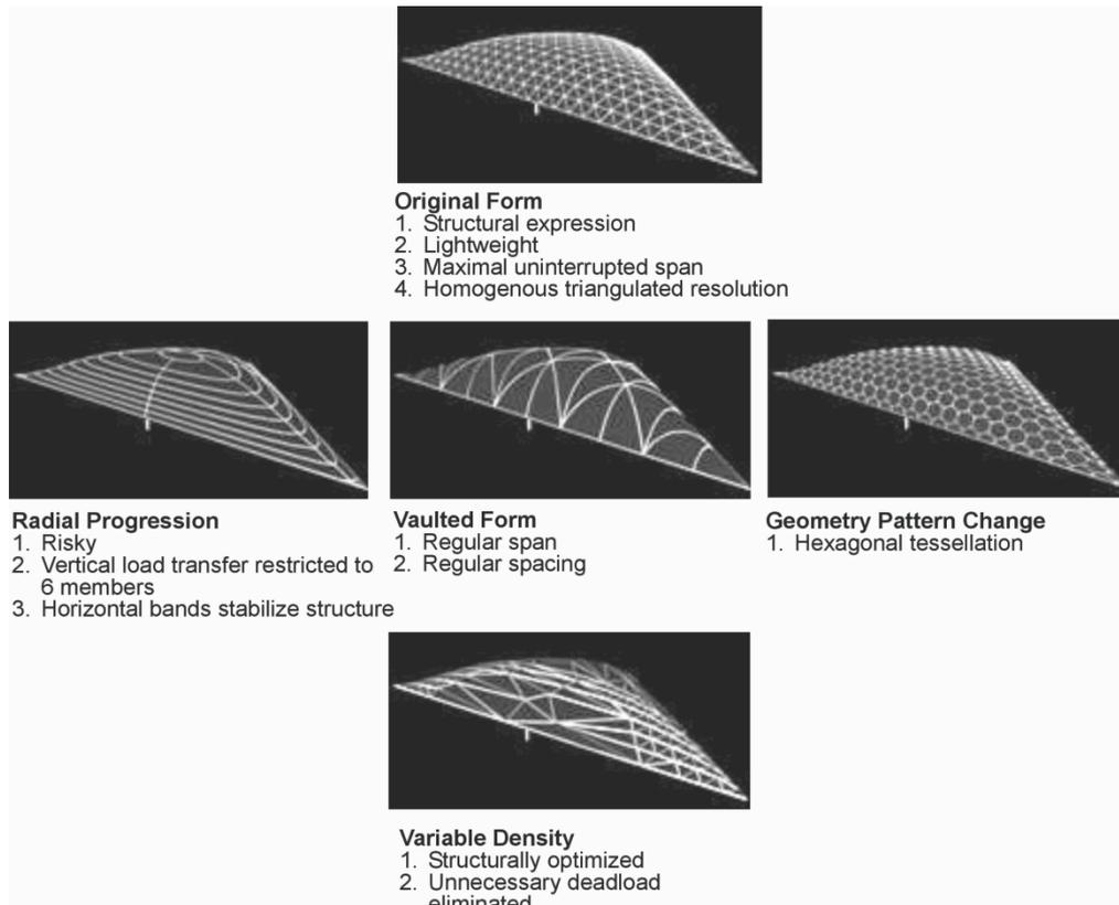
FIG 9: Various structural form alternatives in relation to the architectural and manufacturing constraints
