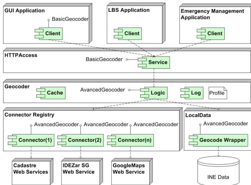
FIG. 7: Layer view of the compound geocoding service and client components.
