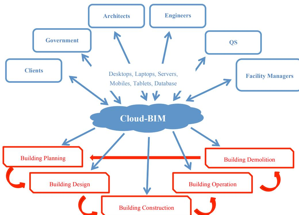
FIG. 1: Cloud-BIM Concept
