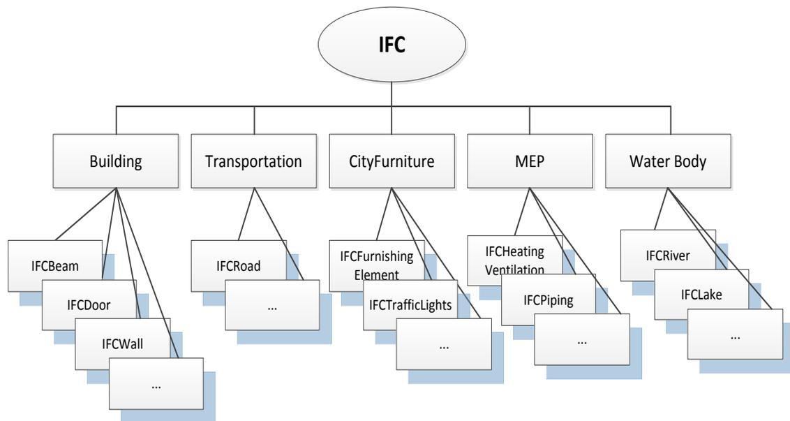
Figure 8: The mapping relationship between IFC and CIM
