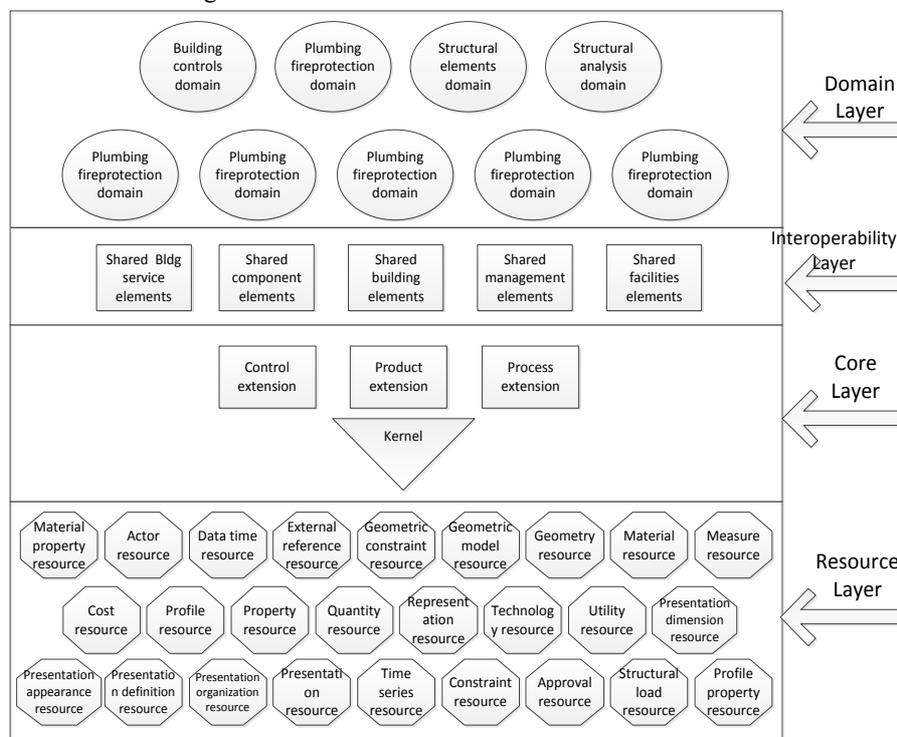
Figure 3: IFC schema
