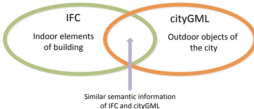
Figure 4: The relationship between IFC and cityGML
