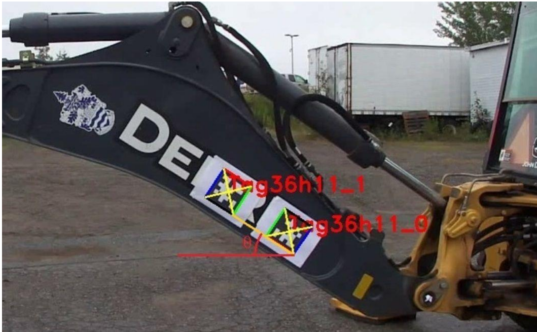
FIG. 3: Markers attached to the boom and the recognized angle
